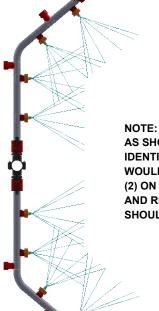
NOTE: THIS RISER CONFIGURATION AS SHOWN CONSISTS OF (2) IDENTICAL RISER SECTIONS, AND WOULD REQUIRE A QUANTITY OF (2) ON THE RISER ORDER. NOZZLE AND RISER SUPPORT QUANTITIES SHOULD BE FOR JUST ONE RISER
